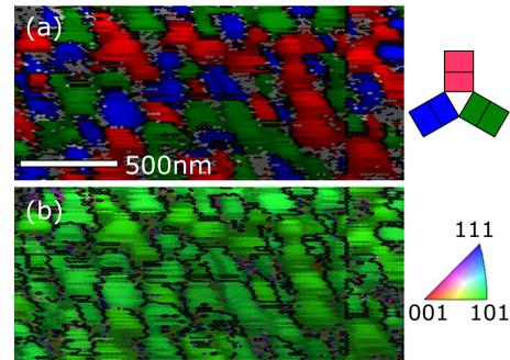
FIG. 3. (Color online) (a) In-plane crystal orientation map (with a  $10^\circ$  tolerance) and (b) inverse pole figure map obtained by EBSD for an Fe/GaN structure grown at HT. Black lines indicate grains boundaries.
