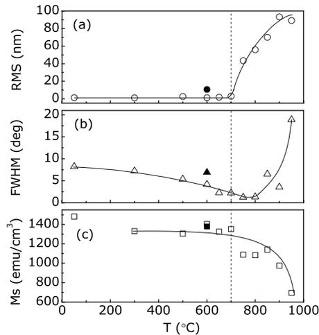
FIG. 5. Dependence of (a) rms roughness, (b) FWHM of Fe{211} reflection, and (c)  $M_S$  of the LT samples on RTA temperature. 50 °C is the growth temperature of the as-grown sample. The solid lines are guides to the eyes. The vertical dashed line indicates the temperature limit for keeping connected Fe films with high  $M_S$ . Filled symbols indicate results for the HT sample for comparison.
