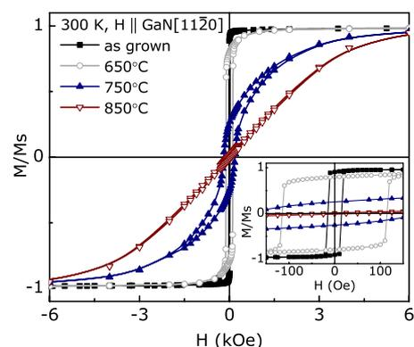
FIG. 4. (Color online) Hysteresis loops obtained at  $300$  K for selected samples from the LT structure. The inset magnifies the low magnetic field range.
