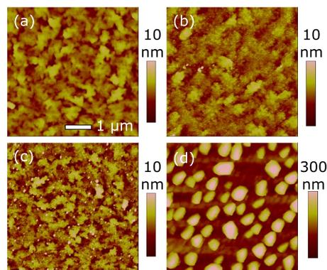
FIG. 1. (Color online) AFM micrographs ( $5 \times 5 \mu\text{m}^2$ ) of (a) the as-grown LT sample and samples annealed at (b) 300 °C, (c) 650 °C, and (d) 850 °C, respectively.
