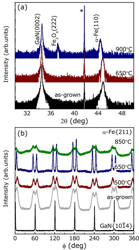
FIG. 2. (Color online) (a) Symmetric x-ray  $\omega$ - $2\theta$  scans of selected samples from the LT structure. The peak labeled with a star is the  $\text{Al}_2\text{O}_3(0006)$  reflection. (b)  $\phi$  scans of the  $\text{GaN}\{10\bar{1}4\}$  and  $\alpha\text{-Fe}\{211\}$  planes.
