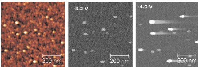
FIG. 1. (Color online) Part of a bias voltage series: Left: Morphology mapping, false color scale is 3 nm. Center: Current mapping of the same area at 3.2 V, color scale is 53.50 pA [nonlinear (Ref. 2)]. Right: Current mapping at 4.0 V, color scale is 100 pA (nonlinear). The morphology does not change during the entire bias series. The striping artifacts are a capacitance effect induced by the preamplifier.
