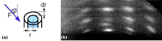
FIG. 2. (Color online) (a) Radial growth of a nanowire having a radius of  $r$ . The flux impinging at a rate of  $F$  is inclined by an angle of  $\varphi$ . (b) RHEED pattern in the  $[\bar{1}10]$  azimuth of sample C. The image was taken at the growth temperature after the MnAs overgrowth.
