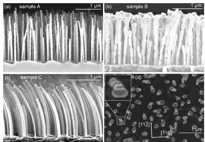
FIG. 1. Scanning electron micrographs of GaAs nanowires enveloped by MnAs on GaAs(111)*B*. The substrate was rotated during growth for [(a) and (b)], whereas it was not for (c). A plane view of sample B is shown in (d). The [ $\bar{1}$ 10] and [ $\bar{2}$ 11] directions of the substrate are indicated. The inset shows an individual nanowire with expanded scales.
