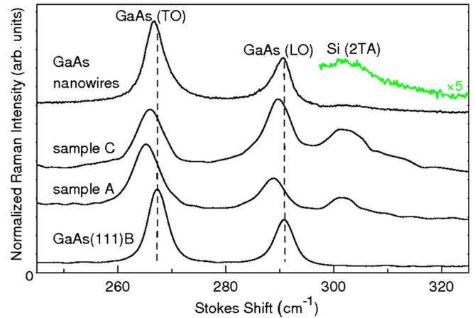
FIG. 3. (Color online) Raman spectra at room temperature from samples A and C, GaAs nanowires, and a GaAs(111)B substrate. The nanowires were placed on SiO<sub>2</sub>/Si substrates. The peaks are associated with the LO and TO phonons in GaAs and the transverse acoustic (TA) phonons (second order) in Si. Curves are offset for clarity.
