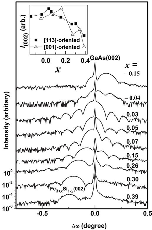
FIG. 1. Normalized skew-symmetric  $\omega$ - $2\theta$  scans of  $\text{Fe}_3\text{Si}/\text{GaAs}(113)A$  near the superlattice (002) reflection. The curves are normalized to the GaAs(002) reflection and are shifted with respect to each other for clarity. The inset shows a plot of intensity of (002) reflection  $I_{(002)}$  as a function of the composition  $x$  for [113]- and [001]-oriented films.
