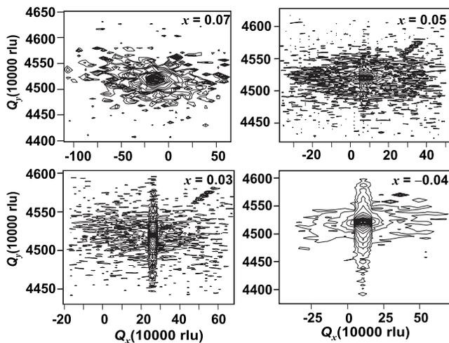
FIG. 2. X-ray reciprocal space maps of stoichiometric  $\text{Fe}_3\text{Si}$  films grown on  $\text{GaAs}(113)A$  substrates for the symmetric and superlattice (113) reflection. The reciprocal lattice unit (rlu) is  $\lambda/2d$ , where  $\lambda$  is the wavelength of  $\text{Cu } K\alpha_1$  radiation and  $d$  is the lattice plane spacing of the corresponding reflection.
