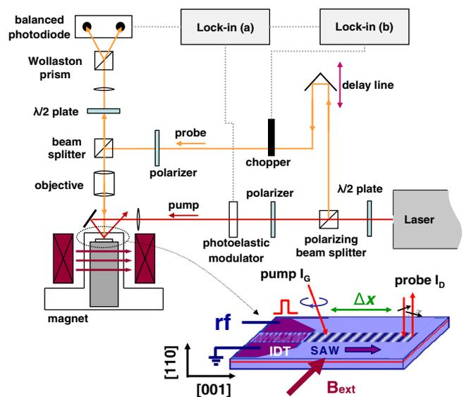
FIG. 1. (Color online) Setup for the detection of acoustic spin transport using TRKR. The IDT launches SAWs propagating along the [001] axis. Spin polarized electrons are excited by a circularly polarized pump beam and detected using a probe beam focused  $\Delta x$  away from the pump.
