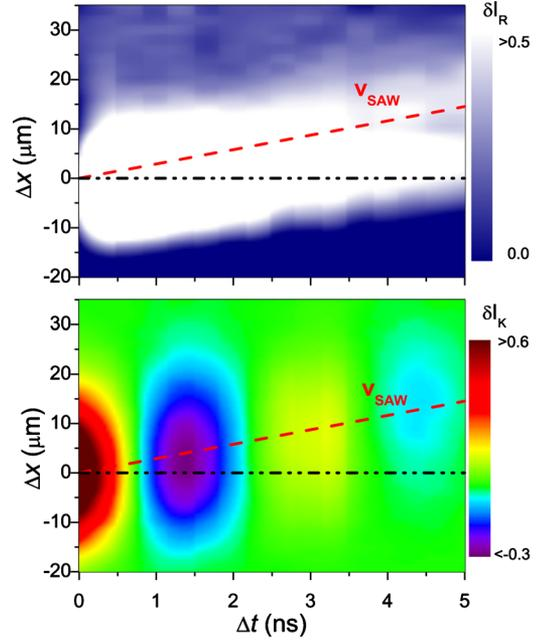
FIG. 2. (Color online) (a) Reflectivity ( $\delta I_R$ ) and (b) Kerr signal ( $\delta I_K$ ) as a function of the delay time ( $\Delta t$ ) and distance ( $\Delta x$ ) between pump and probe pulses under a magnetic field  $B_{\text{ext}}=65 \text{ mT}$  and a SAW power  $P_{\text{rf}}=20 \text{ dBm}$ . The dashed line has a slope equal to the SAW velocity  $v_{\text{SAW}}$ .
