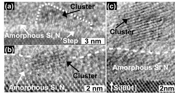
FIG. 3. Cross-sectional HRTEM images of a sample from stage 2 grown on Si(001). The sample is covered by GaN clusters (a) in contact with the underlying Si substrate at a step, (b) embedded in the amorphous  $\text{Si}_x\text{N}_y$  layer, and (c) on top of the amorphous  $\text{Si}_x\text{N}_y$  layer. There is no indication of the defective layer observed in Fig. 2(b).
