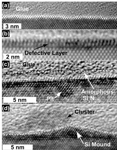
FIG. 2. HRTEM images of different areas of a sample from stage 1 grown on Si(001) [(a)–(d)] cross-sections along  $[110]_{\text{Si}}$  revealing an atomically flat Si area, the formation of a thin crystalline layer, and Si mounds and pits, respectively. The layer in (b) is possibly disordered Si or  $\text{Si}_x\text{N}_y$ , and the clusters in (d) are attributed to GaN.
