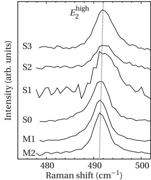
FIG. 2. Raman spectra of the  $E_2^{\text{high}}$  mode for undoped (S0), silicon doped (S1–S3), and magnesium doped (M1, M2) InN nanowires obtained using visible excitation after subtraction of the Si background.
