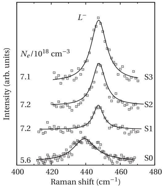
FIG. 3. Line shape fits (solid lines) to the visible Raman spectra of the  $L^-$  phonon-plasmon coupled mode (open squares) for the undoped InN nanowires (S0) and for the Si-doped nanowires (S1–S3). The Si background has been subtracted from the spectra.
