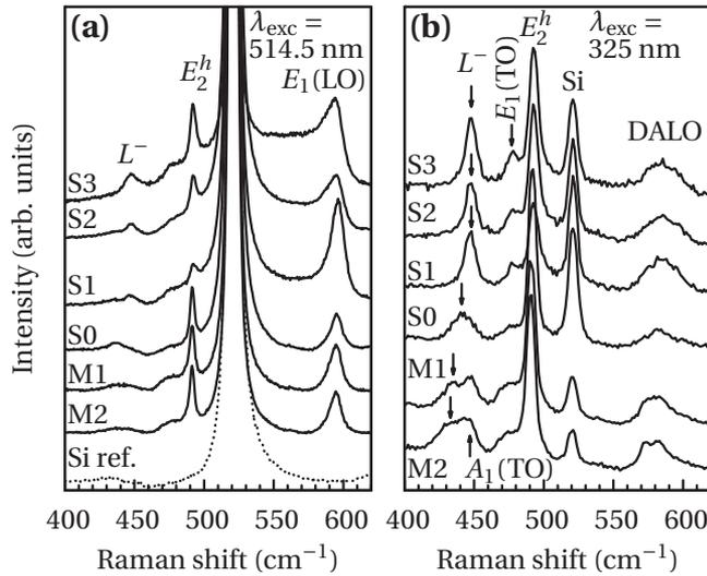
FIG. 1. Raman spectra of undoped (S0), silicon doped (S1–S3), and magnesium doped (M1, M2) InN nanowires obtained using (a) visible and (b) ultraviolet excitation.
