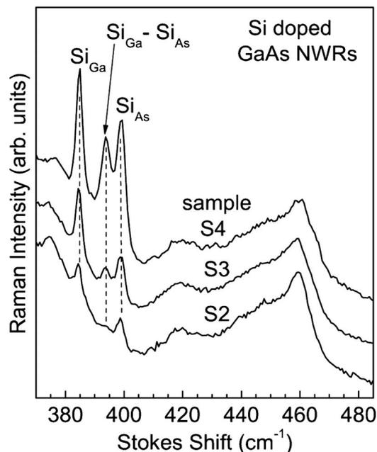
FIG. 2. Low-temperature (77 K) Raman spectra of Si doped samples S4, S3, and S2 excited at a photon energy of 3.00 eV.
