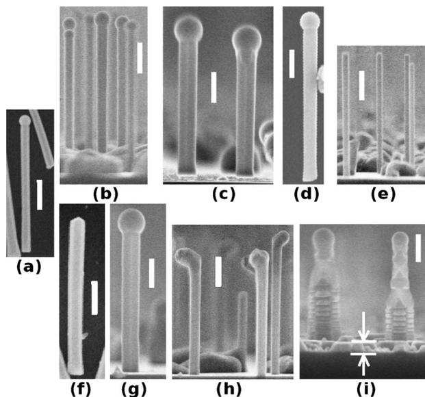
FIG. 1. Scanning electron micrographs of GaAs NWRs from samples R (a), S1 (b), S2 (c), S3 (d), S4 (e), B1 (f), B2 (g), B3 (h), and B4 (i). The scale bars indicate 200 nm. Images (a), (d), and (f) are taken from dispersed NWRs whereas the other images are taken from the as grown samples.
