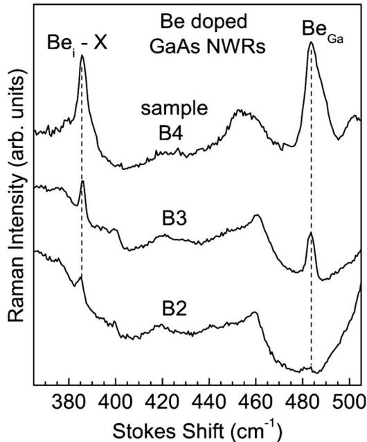
FIG. 3. Low-temperature (77 K) Raman spectra of Be doped samples B4, B3, and B2 excited at a photon energy of 3.00 eV.
