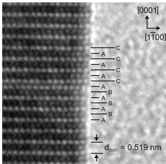
FIG. 2. HRTEM image of a basal-plane SF as marked in Fig. 1. The SF is of  $I_1$ -type and starts on the Aa layer (...ABABACACAC...).
