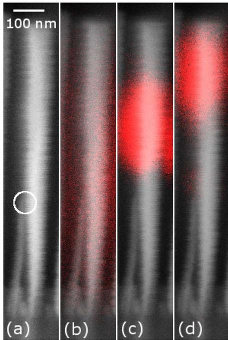
FIG. 4. (Color online) (a) SEM image, [(b)–(d)] SEM and superimposed monochromatic CL images of the same freestanding coalesced NW as shown in Fig. 3. For (b), (c), and (d), the CL detection energy was chosen to be 3.28 eV (ZPL), 3.42 eV ( $SF_1$ ), and 3.47 eV [ $(D^\circ, X)$ ], respectively. The white circle in (a) indicates the contact point between the two freestanding coalesced NWs.
