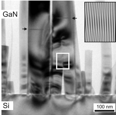
FIG. 1. TEM overview of two coalesced NWs. The black arrows indicate the location of SFs. The white box indicates the location of boundary dislocations just above the contact point. The inset reveals a Fourier-filtered enhancement showing only the  $\{1\bar{1}00\}$  lattice planes to emphasize the edge character of the boundary dislocations.
