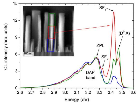
FIG. 3. (Color online) CL spectra recorded at 6 K and excited at the bottom, center, and top of one freestanding coalesced NW. The SEM image in the inset shows the corresponding regions that were analyzed for the CL measurements.
