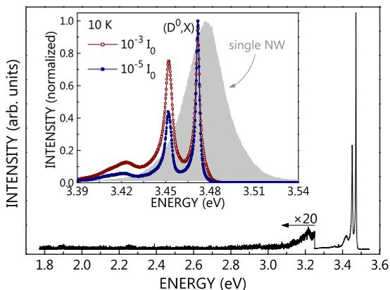
FIG. 2. (Color online) MPL spectrum of the NW ensemble displayed in Fig. 1 at 10 K and an excitation density of  $10^{-5}I_0$ . The inset shows an expanded view of the near-band-gap PL lines at two different excitation densities as indicated in the figure. The shaded area depicts a spectrum of a strained single NW for comparison.
