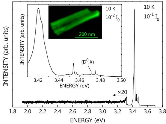
FIG. 3. (Color online)  $\mu$ PL spectrum of the dispersed single NW displayed in the inset at 10 K and an excitation density of  $10^{-1}I_0$ . The inset also shows an expanded view of the near-band-gap PL lines at an excitation density of  $10^{-2}I_0$ .
