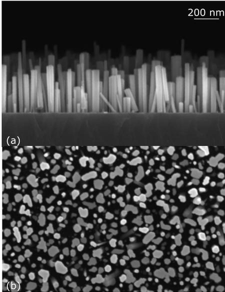
FIG. 1. (a) SEM side view and (b) SEM top view of the as-grown NW ensemble.
