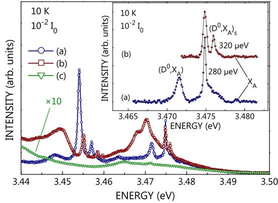
FIG. 5. (Color online)  $\mu$ PL spectra of the single NW displayed in Fig. 3 at 10 K and an excitation density of  $10^{-2}I_0$  taken (a) right after, (b) one, and (c) five months after its dispersion on the Si(111) carrier. The inset shows the first two spectra after background subtraction. The symbols represent the data, the solid lines Gaussian fits to determine the spectral position and linewidth of the individual transitions.
