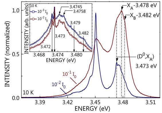
FIG. 4. (Color online)  $\mu$ PL spectra of another dispersed single NW at 10 K and excitation densities of  $10^{-1}I_0$  and  $10^{-2}I_0$ . The position of the most important transitions is marked by dashed lines. Arrows point to the labels of these transitions. The inset shows high-resolution spectra of the near-band-gap PL lines at excitation densities of  $10^{-2}I_0$  and  $10^{-3}I_0$ . All relevant transitions are marked by arrows and their energies are denoted in the figure.
