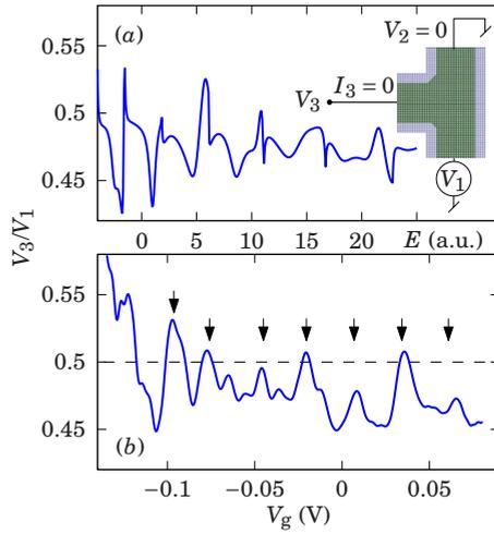
FIG. 4. (Color online) (a)  $V_3/V_1$  ratio vs energy, calculated for a device with asymmetrically rounded corners in the coupling region (see inset). (b)  $V_3/V_1$  data obtained as a function of gate voltage at  $T_e \approx 0.2$  K for  $V_1 = 50$   $\mu$ V (measurement scheme is shown above). Arrows correspond to minima on  $G_{23}$  curve.
