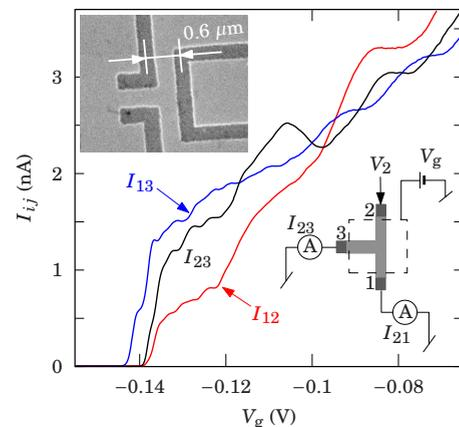
FIG. 1. (Color online) Currents  $I_{ij}$  vs gate voltage  $V_g$  at  $T_e \approx 0.3 \text{ K}$ .  $I_{ij}$  is defined as current flowing from contact  $j$  when voltage  $V_i$  is applied to terminal  $i$  (see the measurement scheme),  $T_e$  is estimated temperature of the electron liquid (lattice temperature was about 0.2 K lower). Upper inset shows scanning electron micrograph of the T-junction device, top metal gate is not visible here.
