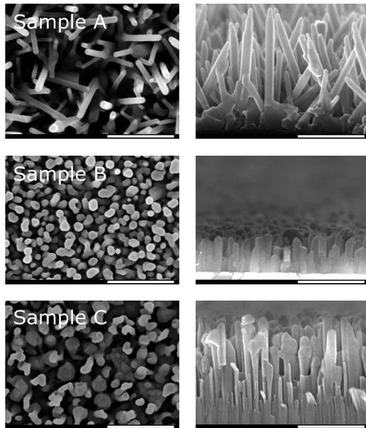
FIG. 1. Topviews (left) and sideviews (right) of as-grown ZnO NWs on Si (top),  $\text{Al}_2\text{O}_3$  (middle), and ZnO (bottom) as obtained by a scanning electron microscope. The scale bars correspond to 500 nm.
