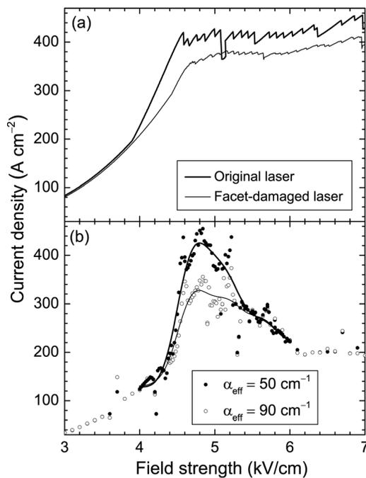
FIG. 4. (a) Measured current density as a function of average field strength for the original (thick line) and two-facet-damaged laser (thin line) at 10 K. The average field strength is calculated by dividing the applied voltage by the thickness of the active region. (b) Calculated current density for two different values of the effective losses. The solid lines are a guide to the eye.
