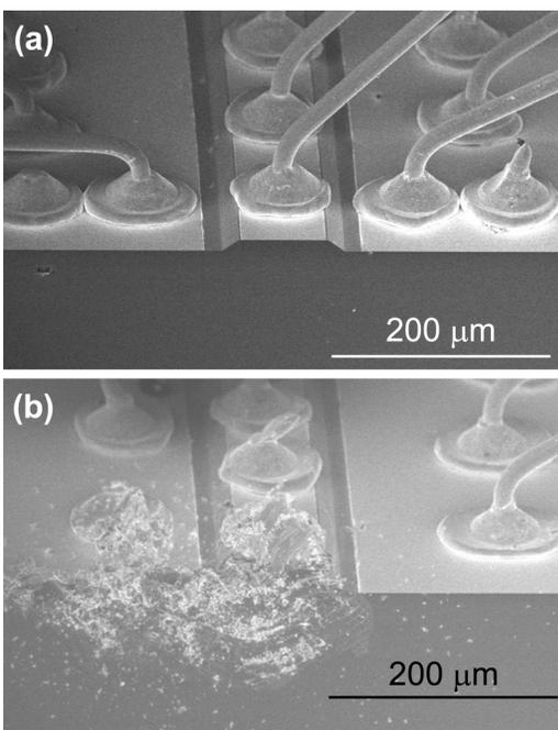
FIG. 2. SEM images of (a) the original facet and (b) the damaged facet with a ridge width of 100  $\mu\text{m}$ .
