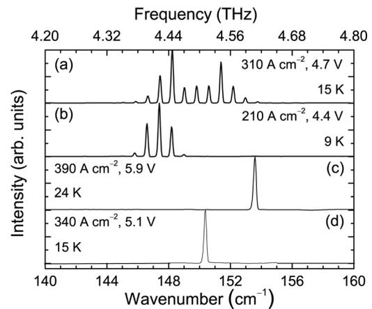
FIG. 3. Cw laser spectra of (a) and (b) the original as well as (c) and (d) the one-facet-damaged QCL.
