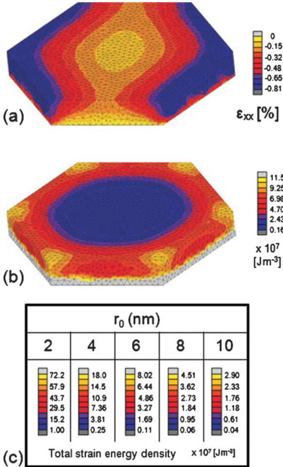
FIG. 5. (Color online) Spatial distribution of (a) the Laplace-pressure-induced strain ( $\epsilon_{xx}$  component) and of (b) the total strain energy density for a NW with a radius of 5 nm. The legend in (c) shows the reduction of the total strain energy density with increasing the radius.
