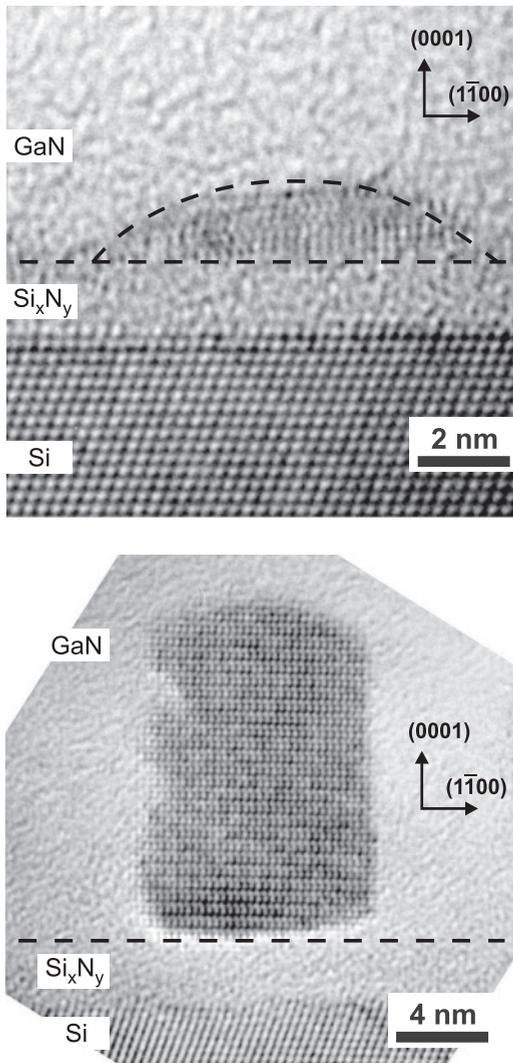
FIG. 2. HRTEM images collected on dedicated samples grown for 7 and 16 min, revealing the following respective GaN island shapes at the onset of the nucleation process: spherical cap-shaped island and NW. The NWs are hexahedral. The shape of spherical caps is outlined for the sake of clarity.
