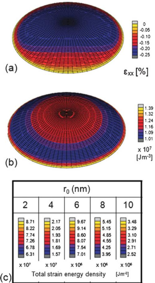
FIG. 4. (Color online) Spatial distribution of (a) the Laplace-pressure-induced strain ( $\epsilon_{xx}$  component) and of (b) the strain energy density for a spherical-cap-shaped island with a radius of 5 nm. The legend in (c) shows the reduction of the total strain energy density with increasing the radius.
