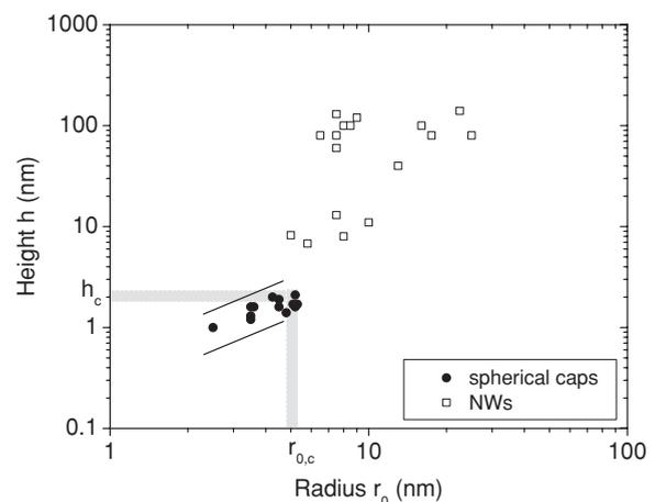
FIG. 3. Height *h* as a function of radius *r*<sub>0</sub> obtained from HRTEM images for the two different shapes of GaN islands as growth proceeds: the spherical caps and NWs are observed on dedicated samples grown for 7, 11, 16, and 24 min and 16 and 24 min, respectively. The gray color regions correspond to the experimental critical height and radius of NWs.
