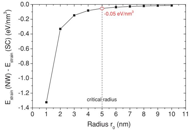
FIG. 6. (Color online) Evolution of the driving force related to strain energy as a function of the island radius. This driving force is defined as the difference between the smallest total strain energy density from FEM calculations of spherical caps with a wetting angle of 42° and of NWs for a given radius.
