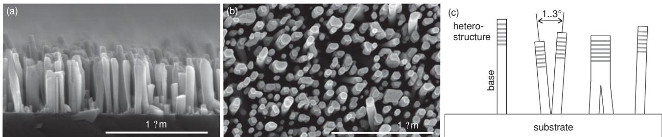
FIG. 1. Scanning electron microscopy (a) side and (b) top views of sample 1 and (c) schematics of the nanowire structure and arrangement.
