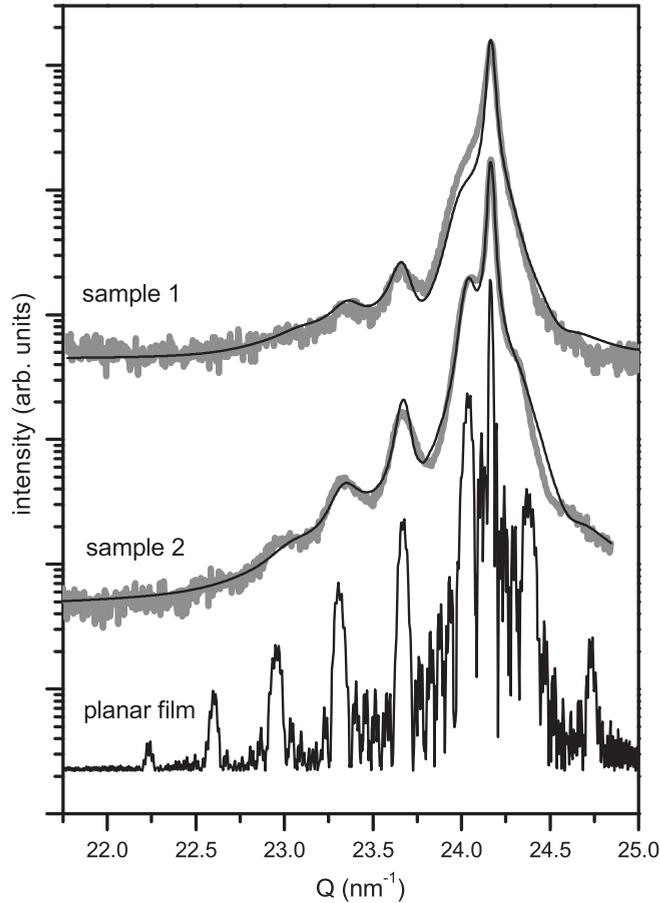
FIG. 2. X-ray diffraction profiles of samples 1 and 2: the experimental profiles (thick gray lines), the calculated profiles (thin black lines), and a calculated profile for an ideal planar heterostructure without fluctuations of the layer thicknesses (bottom line). The curves are shifted vertically for clarity.
