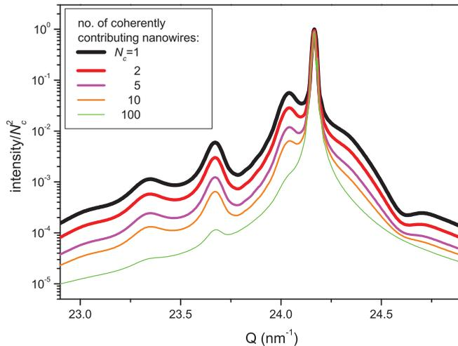
FIG. 4. (Color online) Variation of the diffraction profile with the number of nanowires that coherently add to diffraction.
