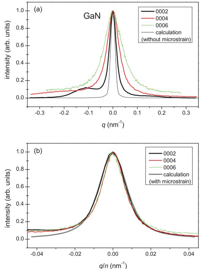
FIG. 3. (Color online) (a) Diffraction peaks of the three subsequent symmetric Bragg reflections from the GaN base layer of sample 2 and (b) the same peaks scaled by the reflection order.
