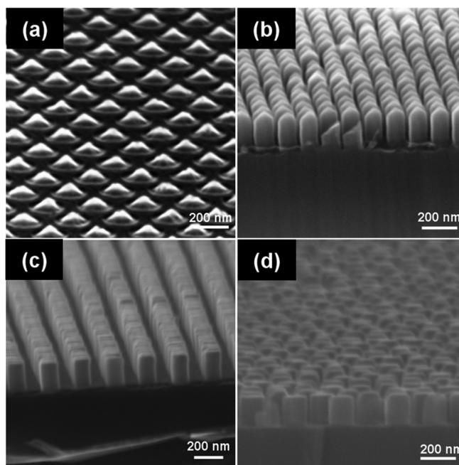
FIG. 1. SEM images of different ordered GaN NC morphologies, grown under the same nominal III/V ratio ( $\approx 3$ ) but different temperatures; (a) 940 °C, (b) 900 °C, and (c) 860 °C. In (d), flat top ordered GaN NCs grown at 900 °C, like (b), but under a nominal III/V ratio of 3.6.
