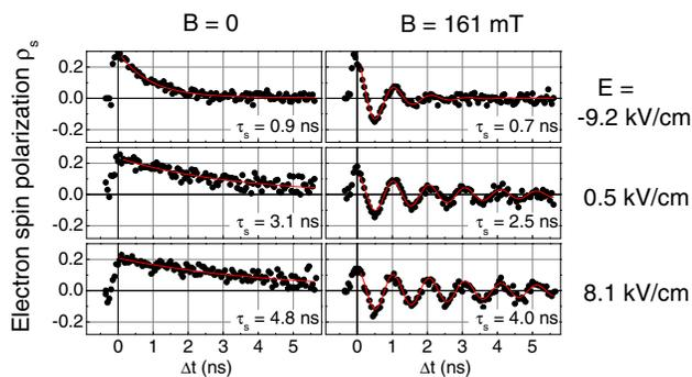
FIG. 6. Temporal evolution of the electron spin polarization  $\rho_s$  in a n-i-p GaAs(111) MQW sample in dependence of the electric field (labelling on the right hand side) measured without (left panels) and with an in-plane magnetic field of  $B = 161$  mT (right panels). The fitting curves (full lines) correspond to single-exponential decay function (left panels) and exponentially damped cosine functions (right panels).  $\tau_s$  denotes the corresponding exponential decay times.
