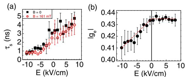
FIG. 7. (a) Electron spin lifetimes  $\tau_s$  measured in n-i-p structures as a function of the electric field without (black squares) and with (red circles) an in-plane magnetic field of 161 mT. (b) Modulus of the electron g-factor in (111) QWs plotted as a function of the electric field strength  $E$ . The dashed line is a guide to the eyes.
