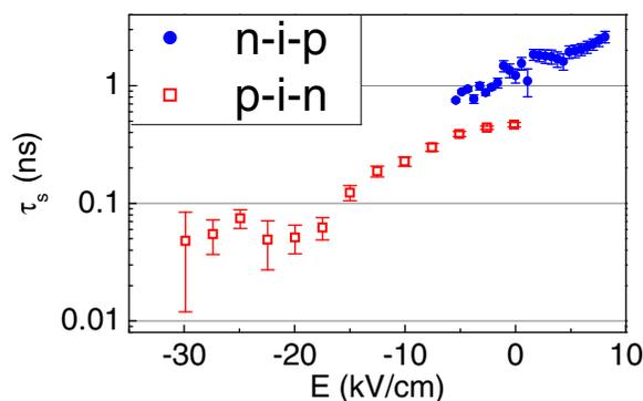
FIG. 8. Electron spin lifetimes  $\tau_s$  deduced from Hanle measurements in p-i-n (red squares) and n-i-p diode structures with (111)B MQWs plotted as a function of the electric field  $E$ .
