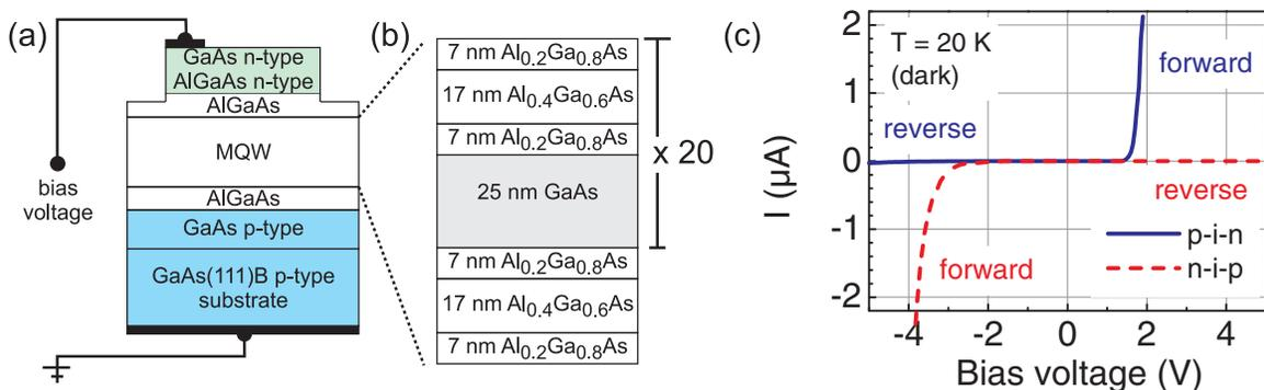
FIG. 3. (a) Layer structure of the n-i-p diodes. The MQW region is illustrated in detail in (b). (c) I-V characteristics of a p-i-n (blue, full line) and a n-i-p (red, dashed line) diode-like structure, taken in the dark at  $T = 20 \text{ K}$ .
