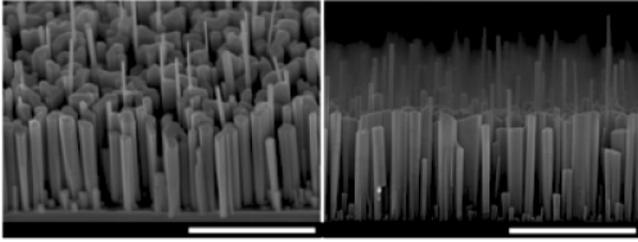
FIG. 1. Tilted (left) and cross-sectional (right) FESEM images of GaN NWs grown for 3 h at a substrate temperature and gallium rate of 780 °C and 0.45 Å/s, respectively. Note that the scale bar is 1 μm.
