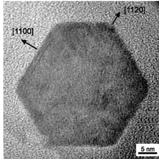
FIG. 2. Top-view HRTEM image of a GaN NW, revealing that the vertical sidewalls are composed of  $m$  planes (i.e.  $(1\bar{1}00)$  planes).
