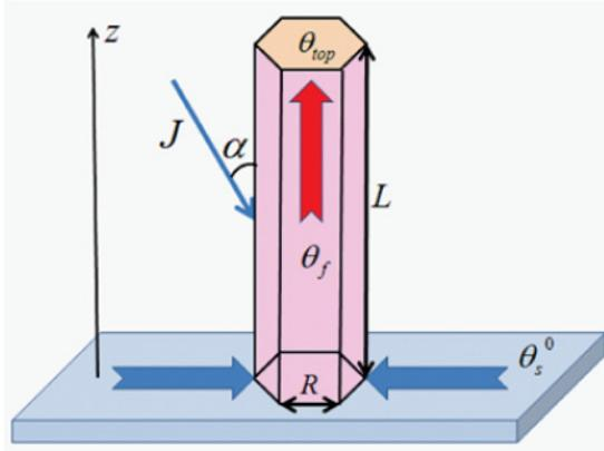
FIG. 3. (Color online) Schematic of the theoretical model for the surface diffusion-induced NW growth in the self-induced approach. The parameters given in the schematic are defined in the text.
