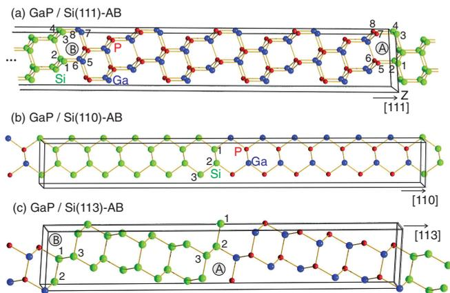
FIG. 1. (Color online) Structure models of the (a) GaP/Si(111)-(2 × 2), (b) GaP/Si(110)-(1 × 1), and (c) GaP/Si(113)-(1 × 1) superlattices. The green, blue, and red atoms correspond to Si, Ga, and P atoms, respectively. A (111) cell in (a) was cut from the left-hand side. A (111) SL consists of type A (P-Si) and type B (Ga-Si) interfaces, whereas both interfaces are equivalent in (b). Substitutional site positions are marked by numbers.
