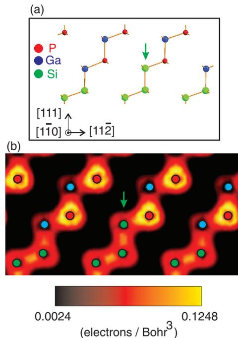
FIG. 4. (Color online) (a) The relaxed atomic plane of the Ga-Si interface of the B-Si-5c structure. The Si substitution site is indicated by a green arrow. (b) Valence electron density cross-sectional map of the corresponding plane. Atomic positions are shown by red, blue, and green spheres for P, Ga, and Si atoms, respectively. There is no significant difference in the valence electron density for the Si substitution site (marked by an arrow).
