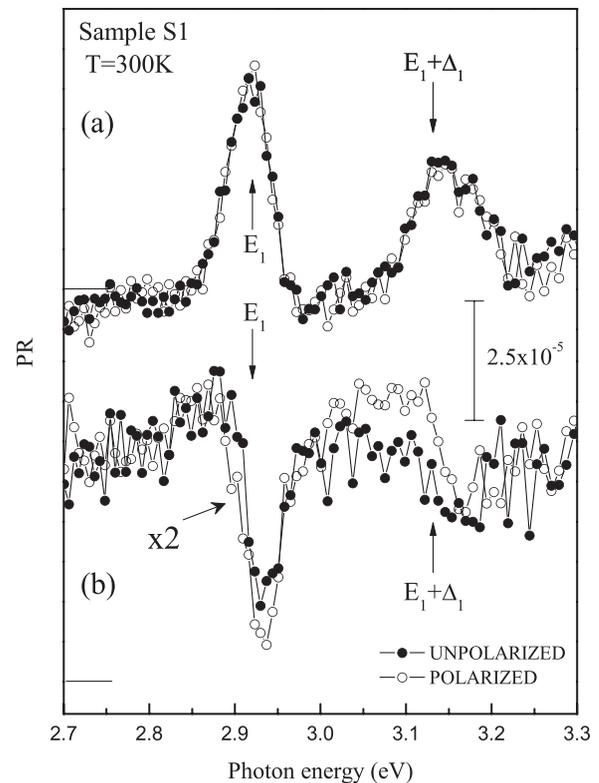
FIG. 2. Photoreflectance spectra for sample S1 (a) before deposition and (b) after deposition of  $\text{Gd}_2\text{O}_3$ . The spectra represented by open and solid symbols were taken with polarized probe light along [110] and with unpolarized probe light, respectively.
