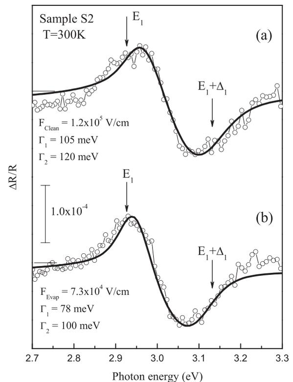
FIG. 5. Photoreflectance-difference spectra of sample S2 (a) before deposition and (b) after deposition of  $\text{Gd}_2\text{O}_3$ . The solid lines represent the fits obtained with Eq. (1) considering the fitting parameters indicated in the figure, where  $\Gamma_1$  ( $\Gamma_2$ ) is the broadening parameter for  $E_1$  ( $E_1 + \Delta_1$ ) optical transition.
