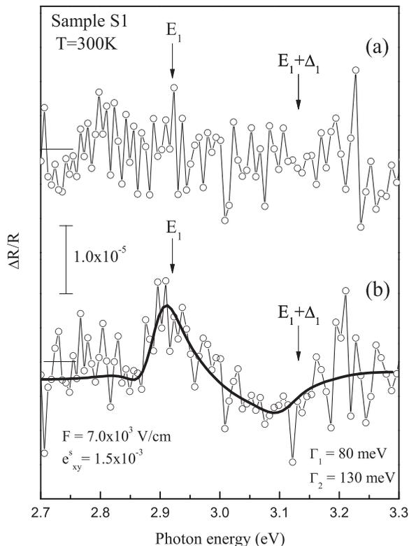
FIG. 4. Photoreflectance-difference spectra of sample S1 (a) before deposition and (b) after deposition of  $\text{Gd}_2\text{O}_3$ . After deposition of  $\text{Gd}_2\text{O}_3$ , a strain is induced on the GaAs surface and a piezo-electric field is created. The solid line represents the fit obtained with Eq. (1) considering the fitting parameters indicated in the figure, where  $\Gamma_1$  ( $\Gamma_2$ ) is the broadening parameter for  $E_1$  ( $E_1 + \Delta_1$ ) optical transition.
