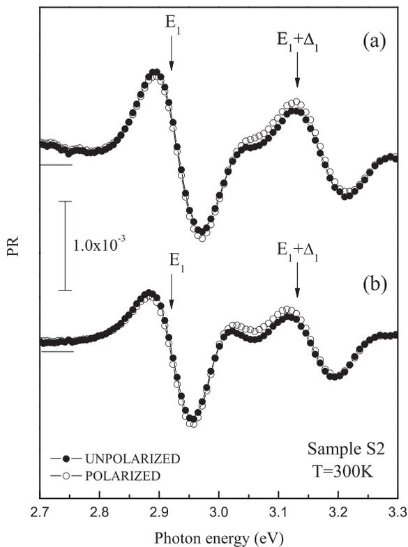
FIG. 3. Photoreflectance spectra for sample S2 (a) before deposition and (b) after deposition of  $\text{Gd}_2\text{O}_3$ . The spectra represented by open and solid symbols were taken with polarized probe light along  $[110]$  and with unpolarized probe light, respectively.
