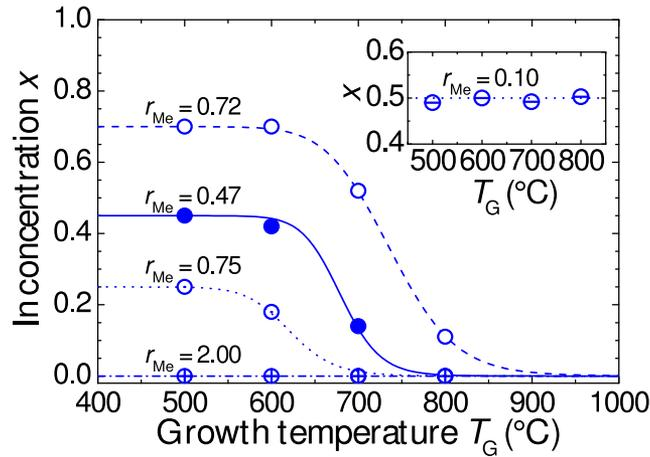
FIG. 3. In concentration  $x$  as a function of growth temperature  $T_G$  plotted for different  $r_{Me}$  and  $x_{nom}$  (see Table I). Inset:  $x$  versus  $T_G$  for  $r_{Me} = 0.10$  (centered discs). The lines are guides to the eye.
