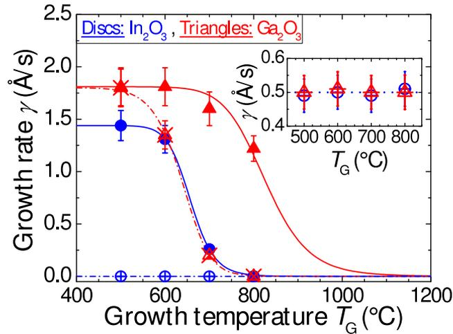
FIG. 4. The pseudo-binary growth rates  $\gamma$  for  $\text{In}_2\text{O}_3$  (discs) and  $\text{Ga}_2\text{O}_3$  (triangles) from the ternary compound  $(\text{In}_x\text{Ga}_{1-x})_2\text{O}_3$  (Figs. 2 and 3) as a function of growth temperature  $T_G$  are depicted for  $x_{\text{nom}} \sim 0.5$  (see text). The symbols correspond to growth parameters indicated in Table I. The lines are guides to the eye.
