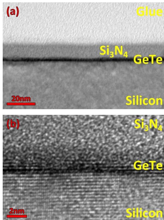
**Figure 2.** (a) Low resolution TEM micrograph of a nominal 1 BL thick GeTe film grown on Si(111)-( $\sqrt{3} \times \sqrt{3}$ )R30°-Sb. (b) Cross-section HRTEM along Si( $\bar{2}11$ ) on the same sample as in (a). These micrographs show that GeTe forms a crystalline and wetting film. The simultaneous coalescence of more than one layer at the same time is also observed.
