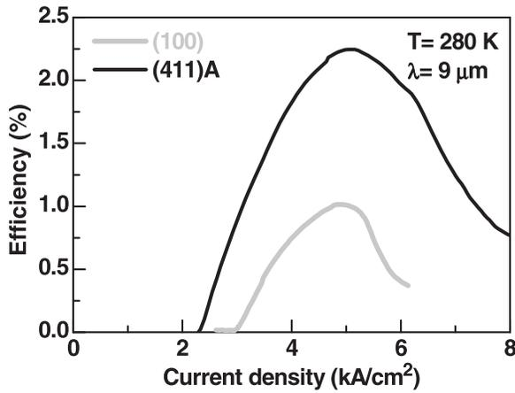
FIG. 2. Power (wall plug) efficiency as a function of the current density compared for the same QCL structures grown on (411)A and (100) oriented InP substrates as indicated. Both lasers were 4 mm long. The lasers grown on (411)A and (100) substrates had  $24.4\ \mu\text{m}$  and  $32.7\ \mu\text{m}$  wide ridges, respectively.
