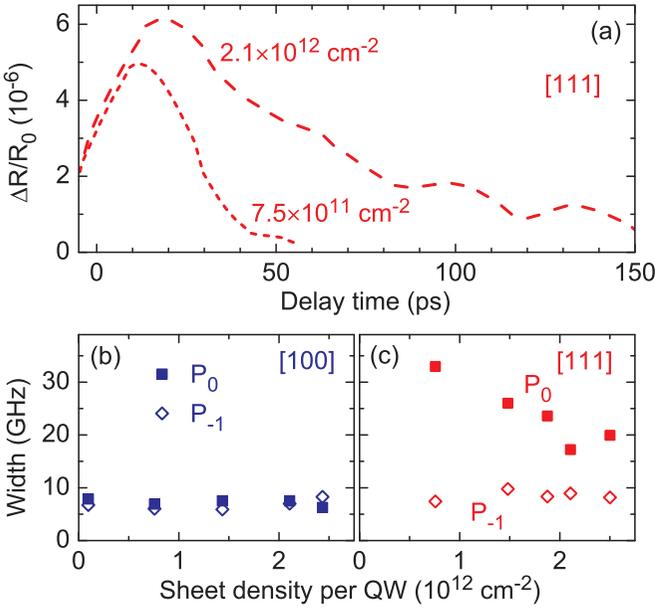
FIG. 3. (a) Envelopes of the  $P_0$  oscillation at 510 GHz in the [111] sample at two different carrier densities. A much faster decrease is observed at lower carrier densities. (b), (c) Corresponding linewidths (FWHM) as a function of carrier density.
