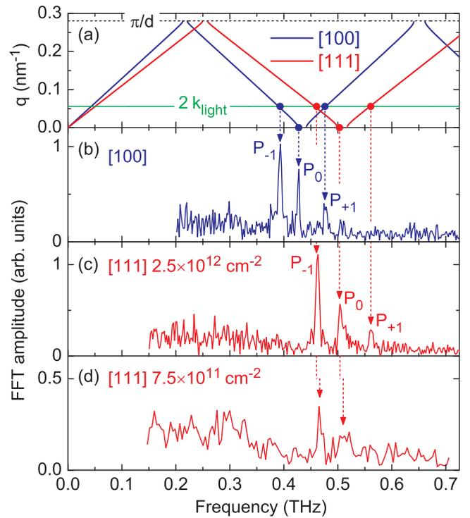
FIG. 2. (a) Calculated dispersion curves of folded longitudinal acoustic phonons for the two growth directions. (b), (c) Spectra of the oscillatory signals from Figs. 1(b) and 1(c). (d) Same as in (c), but for a lower carrier density. The dashed arrows connect the observed peaks to the dispersion curves.
