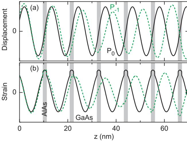
FIG. 4. (a) Displacement of the modes  $P_{-1}$  (dashed green line) and  $P_0$  (solid black line). (b) Corresponding strain. While both the displacement and the stress are continuous at the layer boundaries [Eqs. (2) and (3)], the strain exhibits jumps because of the different elastic constants. The displacement and the strain look identical for longitudinal folded phonons in both directions, [100] and [111], but the strain generates a piezoelectric polarization only in the [111] direction.
